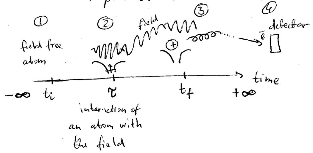
To get analytical solution for ③ we neglect the interaction of the electron and the remaining ion:
