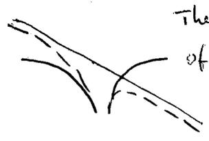
The probability of tunneling is max, because the width of the barrier is smallest.
