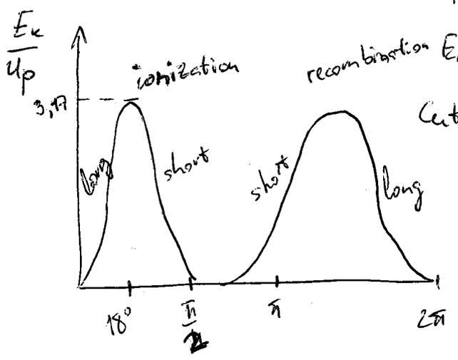
recombination  $E_k = 3,17 U_p$  - maximum kinetic energy at the electron at recombination time.
